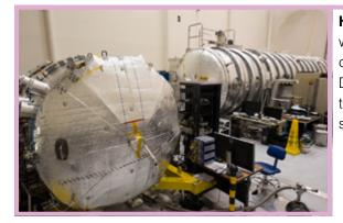
High-Contrast Imaging Testbed (HCIT) Laboratory (JPL): HCIT is the world's premiere facility for demonstrating and advancing space coronagraphs, hosting two vacuum testbeds and one in air, with lasers, DMs, and other optical equipment. The facility was used to demonstrate technology for the RST Coronagraph as well as SAT-funded starlightsuppression technologies that will be needed by HWO.
