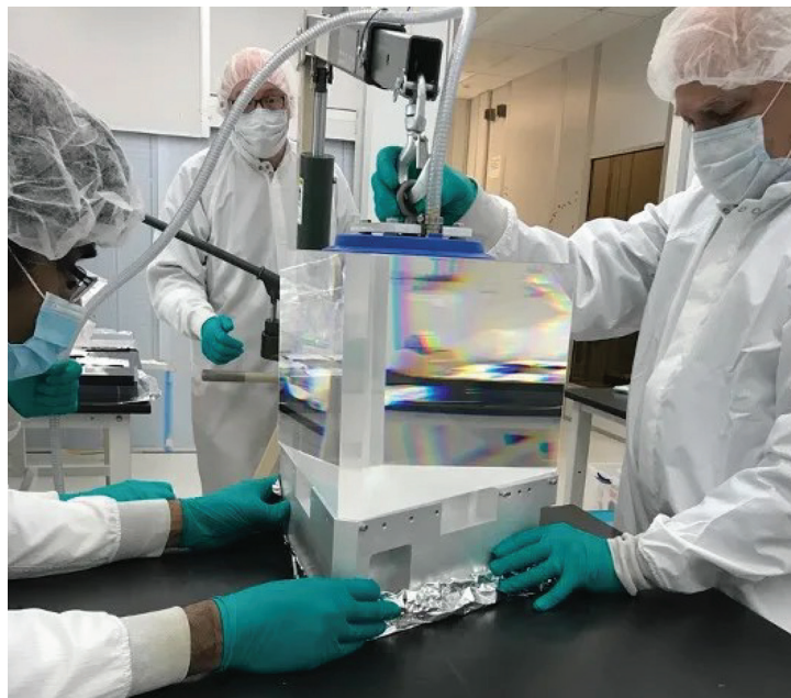
Left to right: Principal Investigator Suvrath Mahadevan, systems engineer Andy Monson, and project manager Fred Hearty install a massive prism into NEID. Image credit: Colin Nitroy
